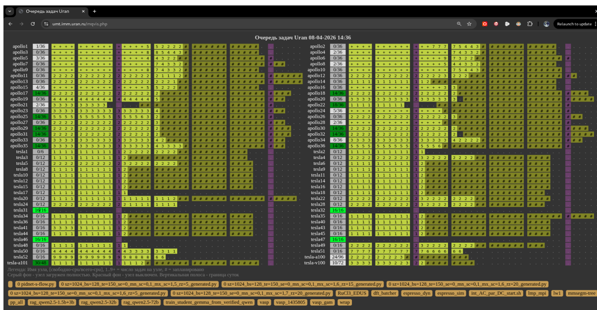
Figure 1. An example of Slurm job queue visualization system output. The visualization program operates in a web environment. The vertical axis displays the node's name and status: [free cores/ total cores]. Status meaning: gray – node is fully loaded, white – node have few free cores, darkgreen – node is half loaded, lime – node is free. Each node is represented by a horizontal bar of cells. Each cell represents one hour. If a cell is yellow, it means that some job is running on that node during that hour. If a cell is darkyellow, it means that some job is scheduled on that hour. 1..9+ represents the number of jobs currently running on the node. The vertical purple bar represents boundary of a day (00:00 am).
