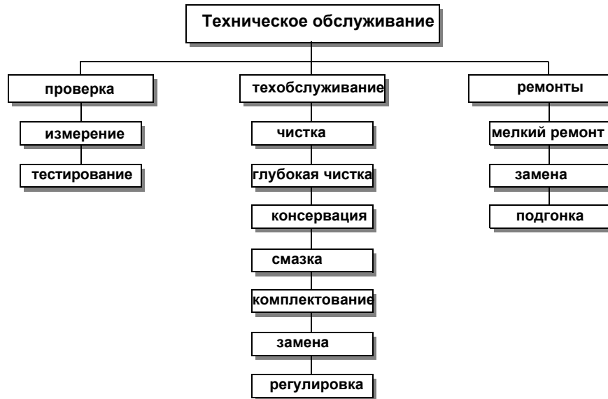
Img. 5-1: Maintenance – Definition according to DIN 31 051
