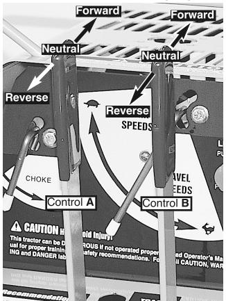
To move *straight* ahead, simultaneously push both Left Track Control (A) and Right Track Control (B) forward.
