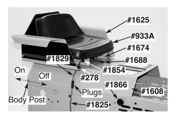
There are **two methods** to remove the Seat Assembly. One is by removing the Assembly as a complete unit (It weighs about 45 lbs.). The second method takes longer but allows you to disassemble the unit into three components that weigh about 15 lbs. each. Both methods are explained below...the choice is yours.
