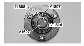
Use your Allen Wrench to tighten the Set Screw ...make sure it's end hits the "V" slot "dead center". With your "open-end" wrench tighten your
