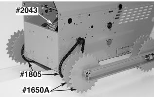
not remove the four nuts on each (Left & Right) #1656 Rear Axle Plate. **NOTE:** loosen the Carriage Bolt "nuts" from inside of body, all others from outside.
