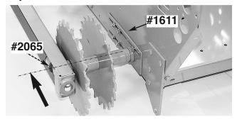
With gloved hands, begin to rotate the Track forward. [TIP: As you rotate the Track, you may want to move the Track Clutch Controls back and forth to relieve any "drag" from the Track Clutch Belts].
