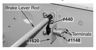
**Disengage** Parking Brake. Remove the two electrical wire plugs from their #1148 Parking Brake Switch and connect a continuity tester to its two terminals.
