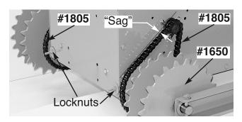
one Locknut 1/4 turn, then go to the other side and tighten the other Locknut 1/4 turn...use this back and forth procedure until both #1805 Drive Chains are reasonably tight...not "bow-string" tight, but about a 1/4" of "sag" in the slack strand when the balance of the chain is taught.
