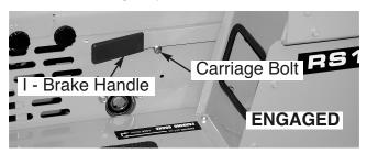
To "engage" Parking Brake, pull Brake Handle up firmly and loop it "up and over" the Carriage Bolt provided...make sure handle edge is on top of Bolt and behind "inside face" of Carriage Bolt.
