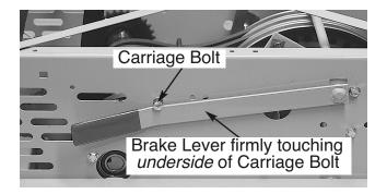
Tighten each of these Brake Assemblies by holding their Adjuster Pin "motionless" with one wrench while tightening their respective Jam Nut securely... a Wrench Slot is provided in each #1792 Yoke (see Photo previous page, lower right).
