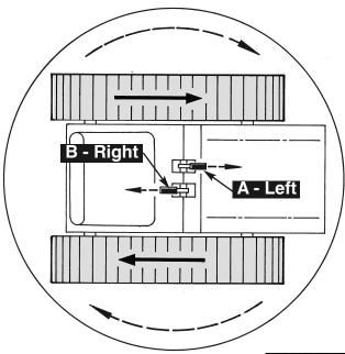
INTRODUCTION: The turn demonstrated (above) is the key to your Crawler's superior maneuverability. It is accomplished with only two controls, the A & B Left & Right Track Controls. The illustrations (below) show how to maneuver your crawler in other turns.
