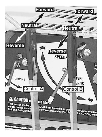
To turn *sharply* to the left, push Right Track Control fully forward...leave Left Track Control in neutral.
