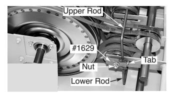
Make sure Belt Release's Lower and Upper Rods are always on the "outside" of the Belts ... **NEVER** inside! Belt Release's Upper Rods should be on **top** and **over** the outside face of its pair of Belts (#1 & #2 on the right; #5 & #6 on the left). Belt Release's Lower Rods should be **below** and **under** the outside face of it's Belts (#3 on the right; #4 on the left).
