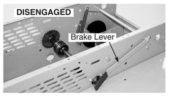
(3) When the Parking Brake Lever is released and put into it's "disengaged" mode (Lever should be free to touch Left Fender) the Parking Switch should be "closed" (the Leaf Spring would have rotated back and away). Continuity light should now be On!
