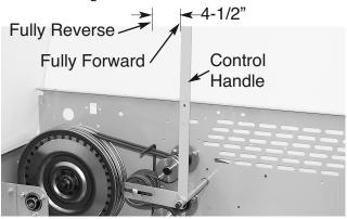
Determine if your Belts are in proper adjustment by measuring the distance of travel (forward to reverse) of each Control Handle. They should travel approximately 4-1/2" when measured at the "furthest end" of their Control Handles. If it is OK, close up your Crawler; **Don't forget** to reconnect #1824 & 1825 Wires & Plugs!
