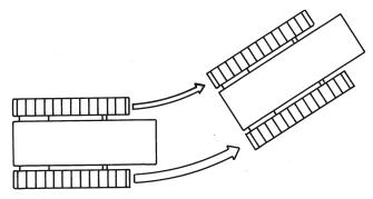
To turn sharply left, push forward on Right Track Control while holding Left Track Control in neutral.
