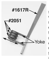
Position each Pulley Assembly (forward or rearward) such that it's respective Control Handle can "rotate" a total distance of 4-1/2" (when measured at the "furthest end" of Control Handle). Complete this adjustment for both Right and Left Pulley Assemblies. When
