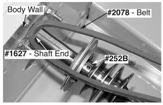
Slip the Track Clutch Belts you are installing through the "slot" you created on the "end" of the appropriate #1627 Upper and #1643 Lower Power
