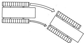
To turn sharply right, push forward on Left Track Control while holding Right Track Control in neutral.
