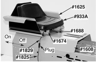
Begin your procedure by parking your Crawler on an open, firm, level surface. Shut off Engine, engage your Parking Brake Lever and dismount. Raise Hood and rotate it fully forward, then remove the #1688 Seat Pin. Remove the #933A Seat & #1674 Mounting Bracket, #1625 Arm Rests, and #1608 Rear Cover. **NOTE:** Disconnect the "mating" #1829 and #1825 Seat Wires at their common Plug.
