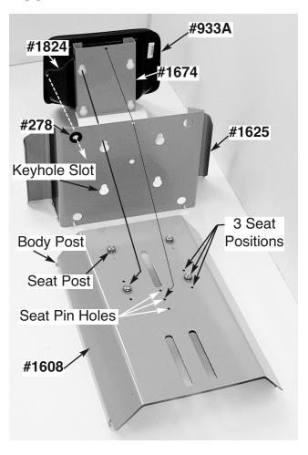
Your Seat & Rear Cover Assembly is made up of three main components: The #1674 Mounting Bracket (with attached #933A Seat) and #1625 Arm Rests mounted to #1608 Rear Cover. They are held together with four "keyhole slots" over four "posts". The "posts" can be located in three different positions to satisfy the operator's "seating comfort".
