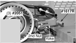
Loosen the 2nd 3/8" Nut holding each of the #2051 three Idler Pulley assemblies in place on their respective #1617R & 1617L Right & Left Control Handle Assemblies. Loosen, so each Pulley Assembly (containing three #2051 Idler Pulleys each) can slide forward and rearward in its respective Yoke.
