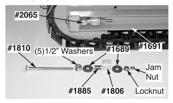
From "outside" the Crawler's body, fully loosen (but do not remove) the five nuts on each (Left & Right) #1611 Front Axle Plate. Slide #2065 Axle fully rearward.
