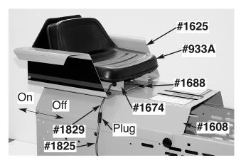
Begin your procedure by parking your Crawler on an open, firm, level surface. Shut off engine and engage Parking Brake. Open Hood and swing fully forward. Remove #1688 Seat Pin. Remove #933A Seat & #1674 Mounting Bracket, #1625 Arm Rests, and #1608 Rear Cover. **NOTE:** Be sure to disconnect the "mating" #1829 and #1825 Seat Wires at their common Plug.
