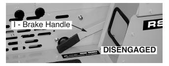
Disengage Parking Brake (I); Fully raise all Attachments to recommended traveling heights.
