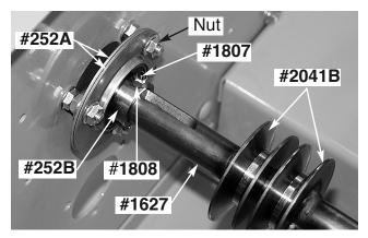
Using the proper sized "Allen Wrench" to hold the #1807 Set Screw, take a proper sized "open end" wrench and turn the #1808 Locking Jam Nut two full turns "counter-clockwise". Then use the Allen Wrench to completely remove this "set screw & nut" assembly...save for reinstallation.
