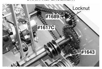
Loosen the Locknut securing the #1689 Idler Sprocket and slide this assembly forward. "Work" the now loose Chain around so the Connector Link is convenient to work on. Remove the Chain Connector Clip and remove the Connector from the Chain. Remove the Chain.
