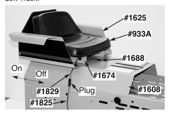
Begin your procedure by parking your Crawler on an open, firm, level surface. Shut off Engine, engage your Parking Brake Lever and dismount. Raise Hood, fully rotate it forward, remove #1688 Seat Pin. Then remove the #933A Seat & #1674 Mounting Bracket, #1625 Arm Rests, and #1608 Rear Cover. **NOTE:** Be sure to disconnect the "mating" #1829 and #1825 Seat Wires at their common Plug.
