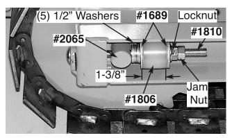
By rotating clockwise the Locknut you mounted to end of each #1810 Tension Bolt, draw the Locknut and associated #1689 Washer (on each Tension Bolt's end) against its respective #1806 Spring such that each Spring is compressed to a total length of 1-3/8" (measured from inside Washer to Washer).
