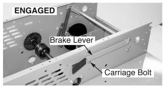
(2) When the Parking Brake Lever is pulled "upward" and looped "up and over" the Carriage Bolt
