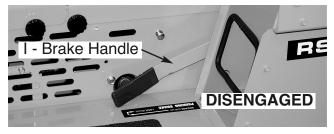
To "disengage" Parking Brake, reverse the above procedure and allow Brake Handle to rest on Fender.
