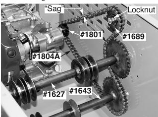
Check your #1804A Engine Drive Chain. Pull up on the recoil starter rope to "tension" the Chain and create slack (sag) in the Chain portion going from #1801 Engine Sprocket to #1689 Idler Sprocket.
