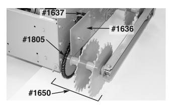
Open Hood and swing fully forward; remove #1688 Seat Pin. Remove Seat & Bracket, Arm Rests and Rear Cover. Remove the #1636 Right & Left Chain Guards from left and right sides of Crawler.
