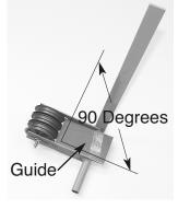
NOTE: as you tighten the (above) Locknuts you must keep the Pulley Assemblies at a 90 degree angle to the Yokes in each Control Handle assembly. Using a "homemade" sheet of metal, wood, etc. (approximately 3-1/4" x 6") as a "guide" is a big help in holding this angle!
