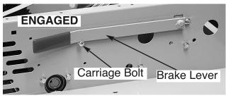
**NOTE:** In the process of making Brake adjustments, try to keep *both* Brakes synchronized with each other for even braking! CHECK WITH FACTORY IF YOU HAVE ANY QUESTIONS REGARDING YOUR BRAKE ADJUSTMENTS!
