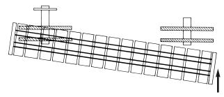
Loop the forward end of the Track around the Inner & Outer Sprockets of Front Idler engaging the Track's Inner Chain between the Inner & Outer Sprockets of the Front Idler.
