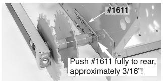
Using a "flat-nosed" punch and hammer, push the #1611 Front Axle Plate (located on both sides of Body) rearward till it hits a solid stop. **NOTE:** in the work done in steps above, this Plate may have already worked its way rearward. To check, push Plate forward from the rear, then push it back the required 3/16" distance.
