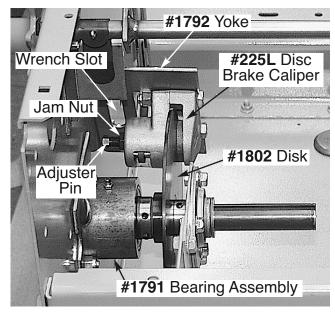
With Brake Lever firmly touching *underside* of Carriage Bolt, set *each* Brake's tension by rotating it's Adjuster Pin *clockwise* until the the Pulleys on each side are not able to be *easily* rotated by hand.
