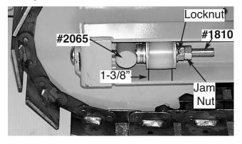
If your Springs have lost this 1-3/8" dimension, or you have just replaced a #1806 Spring or broken #1810 Tension Bolt, follow this procedure:
