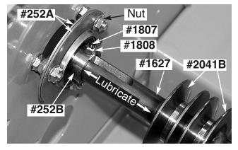
Take original #1807 Set Screw & #1808 Nut "assembly" and thread it into its original threaded hole of bearing...rotate the #1627 (or #1643) Shaft within the bearing to align the end of the #1807 Set Screw with its mating "V" slot in shaft's end.
