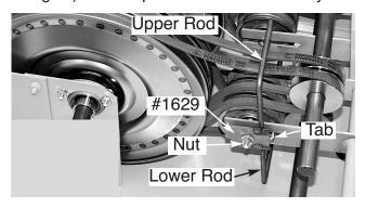
Replace both #1629 Belt Releases using original nuts to secure. **NOTE:** "TAB" goes forward on both sides.
