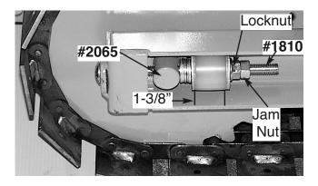
When satisfied, mount a Jam Nut to remaining ends of each #1810 Tension Bolt. Hold each Locknut with a "thin profile" 3/4" open end wrench, and tighten each Jam Nut with a 3/4" box wrench ...tighten securely!
